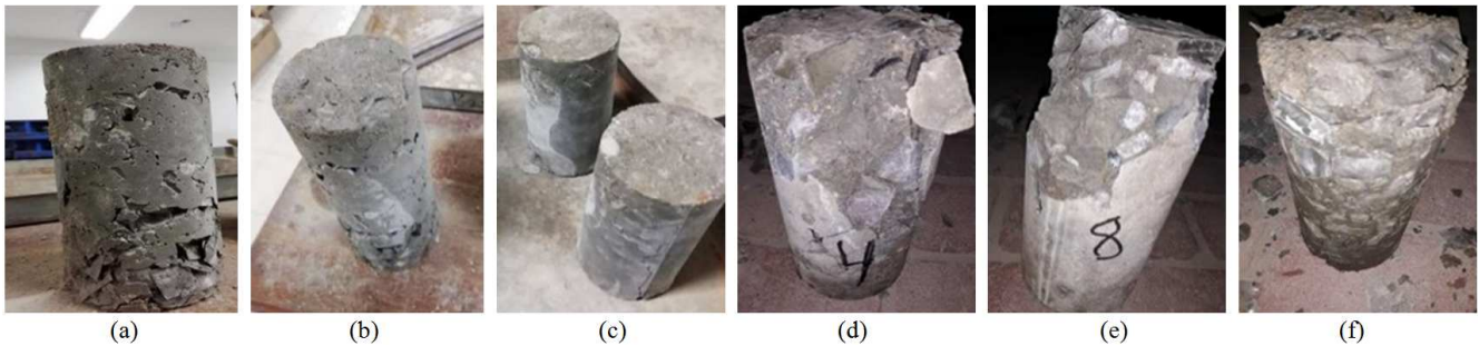
Figure 2. Photographs of specimens (a) CSP15, (b) CSR15, (c) CSG30, (d) Failure of CSR30 (Type 1) at crushing, (e) Failure of CSG15 (Type 4) at crushing and (f) Failure of CSR15 (Type 5) at crushing.
