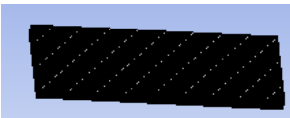
Figure 12. Surface mesh for the plate without weld.
